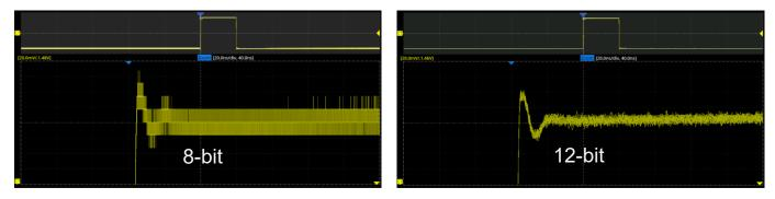
12-bit resolution shows you more details and less noise on the waveform.
